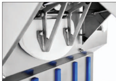
Discharge outlet of PSS SM
