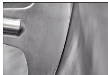
The minimum space between the mixing paddles and the hopper wall
