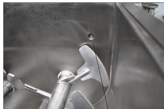
Dosing hole for water dosing
